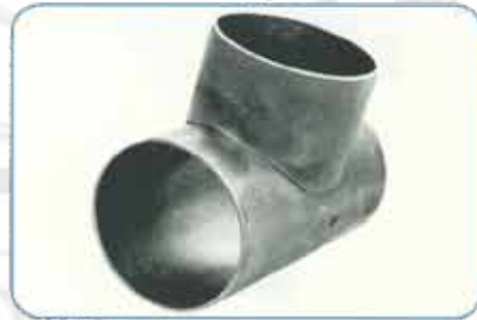
Ø mm 180 tube with 5 mm thickness groove at 90°, carried out with single-head cutter. Cycle time: 20 seconds
