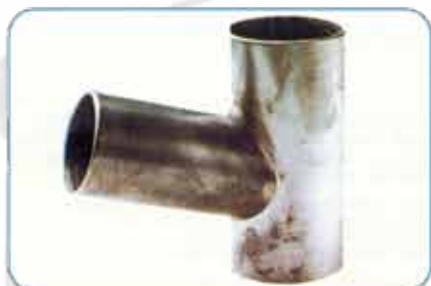
Ø mm 60 tube at 40° coupled to Ø 90; work carried out in 6 seconds
