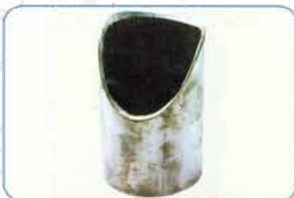
Ø mm 60 tube with groove inclined at 45°, carried out in 5 seconds with double-head cutter
