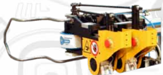
Capacity of minimum space under the bending head for right and left bending, completing the part without requiring off-line bending
