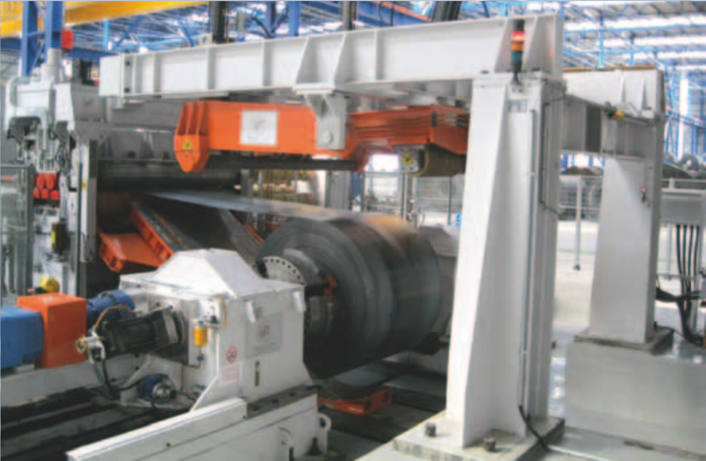
▲ C.T.L. 2100x1,5÷12mm (Decoiler 32 ton)
