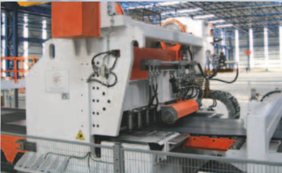
◀ C.T.L. 2100x1,5÷12mm (Flying Shear)
